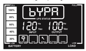
Step 2: The flickering figure would change to "120" after pressing the SELECT-button three times again.
